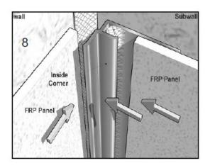
Apply a continuous bead of silicone sealant in the corner and in the Inside Corner PVC Trim Molding channel. Secure Inside Corner PVC Trim Molding to cover bead. (see illustration 8)
