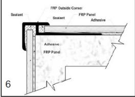
In areas of higher moisture conditions, PVC Trim Molding and FRP Panels must be sealed with Marlite brand Silicone Sealant to ensure a watertight seal. (see illustrations 3 – 6)
