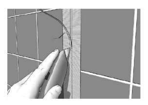
After adhesive sets, removed nails and apply a 2" or wider strip of masking tape over the joint. Trim out groove with a sharp utility knife using the panel edges as guides.
