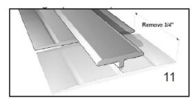
Apply a continuous bead of silicone sealant to both Division Trim Molding channels. Slip under preceding FRP Panel and secure to sub wall. Then, continue with the next FRP Panel. (see illustration 10)
