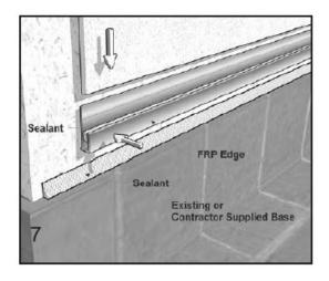
Curb must be installed first. Apply a continuous bead of silicone sealant to the top of curb or floor line and in the PVC Trim Molding channel. Set Edge Trim Molding in place and fasten to the sub wall. Slip FRP Panel into Edge Trim Molding. Allow for 1/8" expansion space and sealant "squeeze-out". Execute similar application at ceiling line. (see illustration 7)
