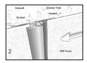
Do not fit panels too tightly into Trim Molding. Allow a 1/16" space in all channels for panel expansion after installation is completed. (see illustration 2)
