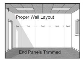
For a balanced appearance, establish a center line of area to be covered and work toward corners. (see illustration 1)
